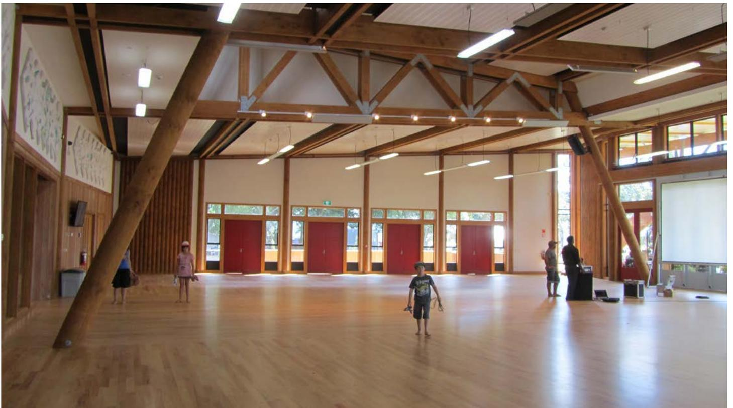
Te Wharehou O Tuhoë uses world first TTT MultiPole structural components in the new iwi and civil defence headquarters located in Taneatua, New Zealand. This project utilised TTT MultiPole Uglie foundation piles, and TTT MultiPole UniLog columns, diaphragm floor panels, and post-tensioned shear wall panels.
